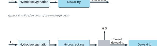
Figure 4. Simplified flow sheet of sweet mode HydroFlex™.
