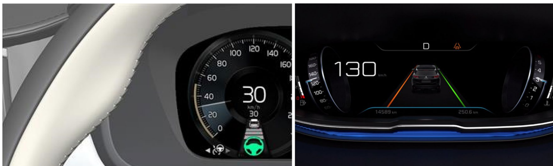
Fig. 7 Dashboard display for Volvo V90 Lane Keeping System (left) and Peugeot 3008 Lane Keep Assist (right). The red lane line on the Peugeot screen indicates that the driver is steering too close to the
