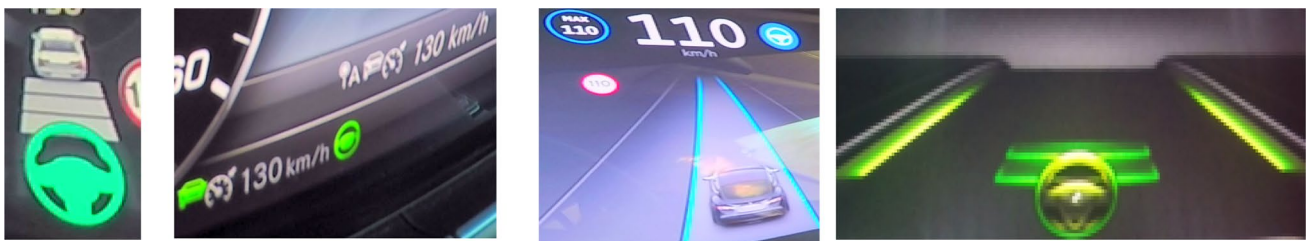
Fig. 1 The Volvo S90, Mercedes E Class, the Tesla and BMW 7 Series indications of activated steering (in the Volvo case without ACC) and proper detection of road markings (Photos copyright UTAC CERAM and FONDATION MAIF)
