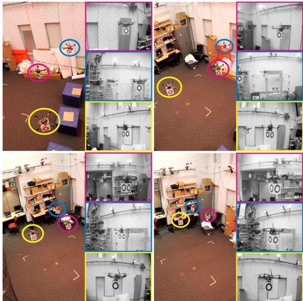
Fig. 24 Experiment with a swarm of 3 MAVs controlled by the feasible FSS rules
