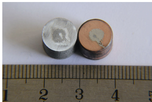
Fig. 2. Appearance of an uncombined Cu/Al couple bonded at a temperature of 550°C for 10 min.
