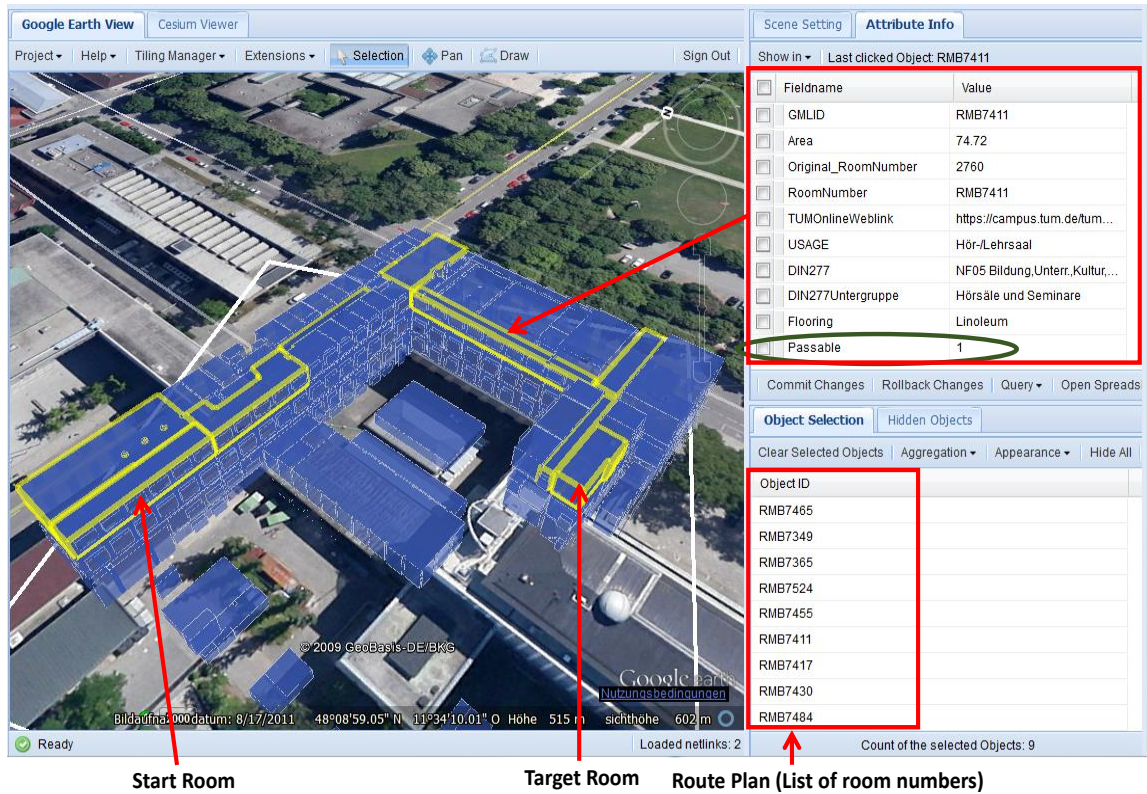
Fig. 6.47 Route plan (with all the semantic and geometric information of the route) from the start room to the target room based on the main network model provided by the building administrator.
