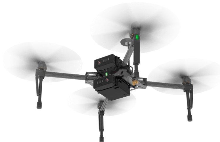
Figure 5: Baseline Matrice 100 UAV with dual batteries. Image sourced from DJI (2019)
