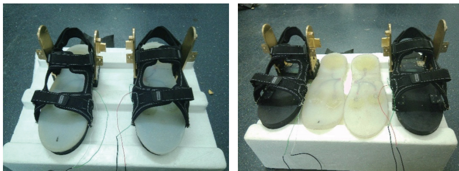
Fig. 8. (Color online) Overall structure of force-sensing shoes.
