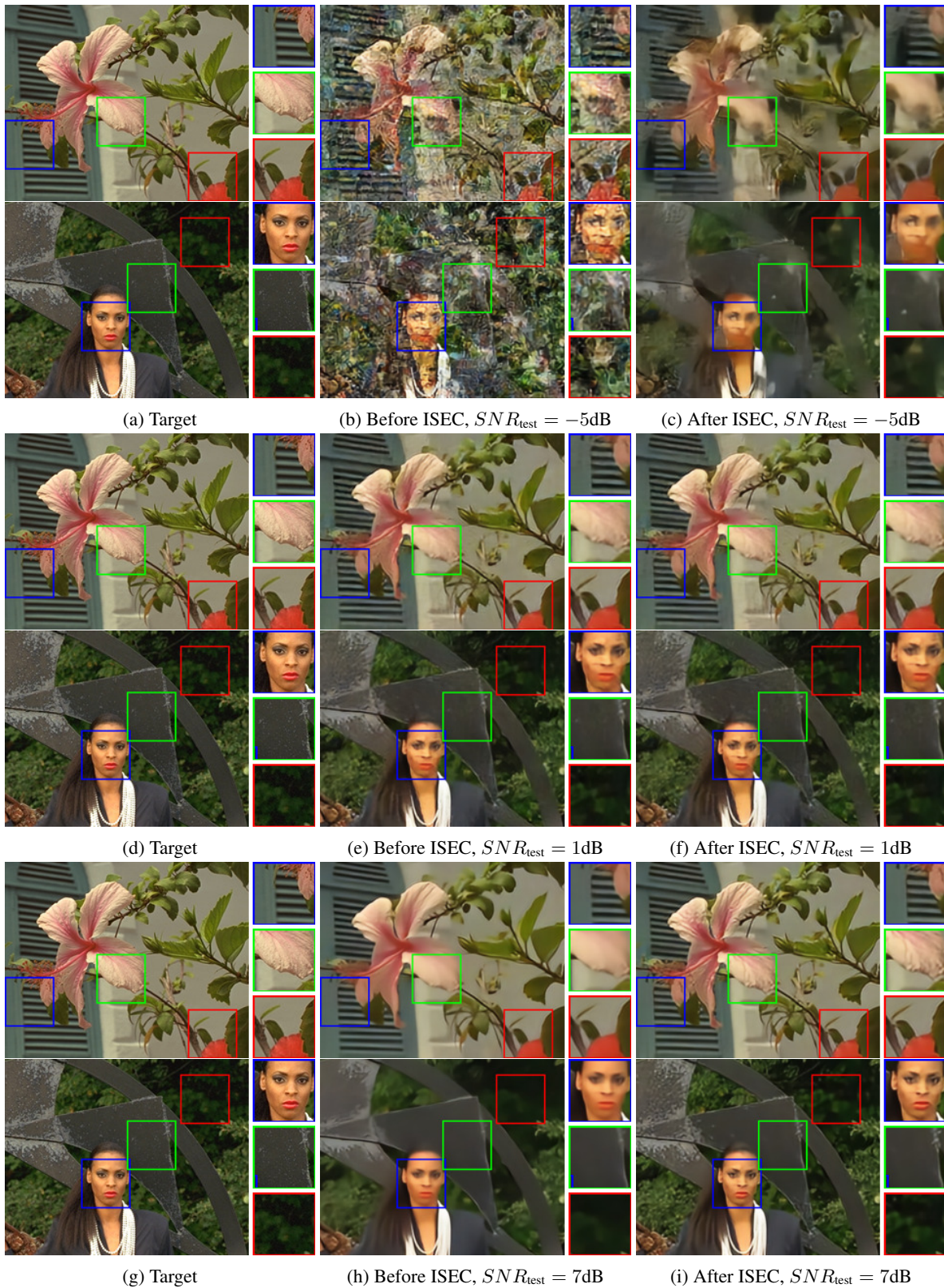
Figure 18: Before and After ISEC on Kodak images using SNR_{train}=1\text{dB} model on CPP=1/16 .
