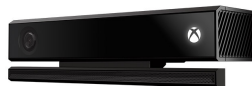
Fig. 1. Kinect version 2 used for multimodal interaction with the robot using voice and gestures
