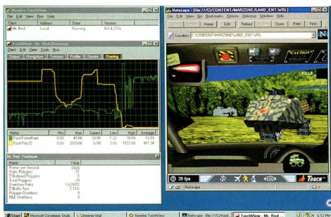
Among the package's more powerful tools is Torchview, which provides realtime graphs of such things as frame rate and polygon count, so trouble spots can be found quickly
