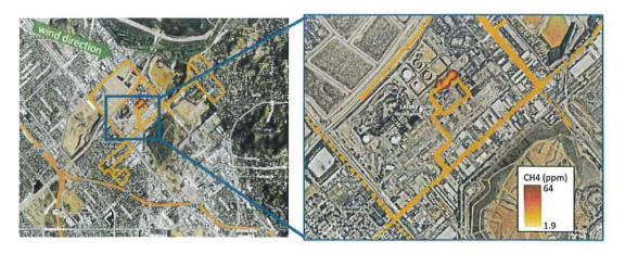
Map showing measurements near the LADWP Valley Generating Station. Elevated levels are results from samples taken on site. (August 27, 8:30am-12pm)
