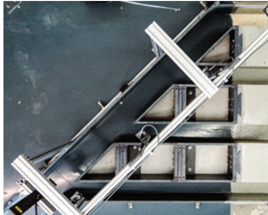
Figure 4. Extract of an open tunnel system model with modular design at RWTH Aachen University. Photograph: Elena Pummer.
