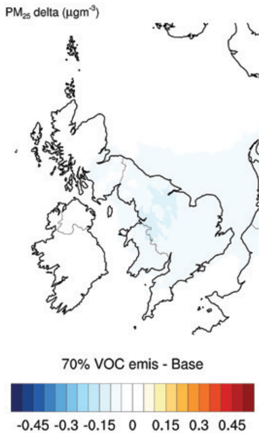
Figure 15: Change in PM 2.5 (µg m -3 ) simulated by the EMEP4UK model for 70% of UK anthropogenic NMVOC emissions (i.e. 30% emissions reduction).
