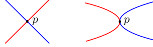
Figure 1: Left: At an A_1 singularity, two branches of the curve intersect transversally. Right: At an A_{2k+1} singularity with k > 1 , the tangent lines of the two branches at the intersection point coincide.
