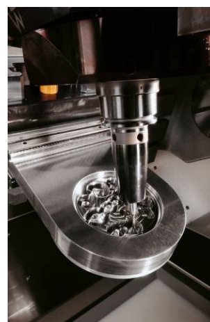
Fig. 6 Metal pieces manufactured by a dynamic high-precision machining centre with five axes
