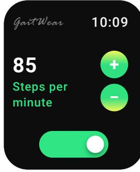
**Figure 7.** A screenshot from GaitWear, a simple smart watch application that produces the Haptic 1P1W cue out in-the-wild. This is enabled or disabled via the toggle widget or two subsequent wrist flickers.
