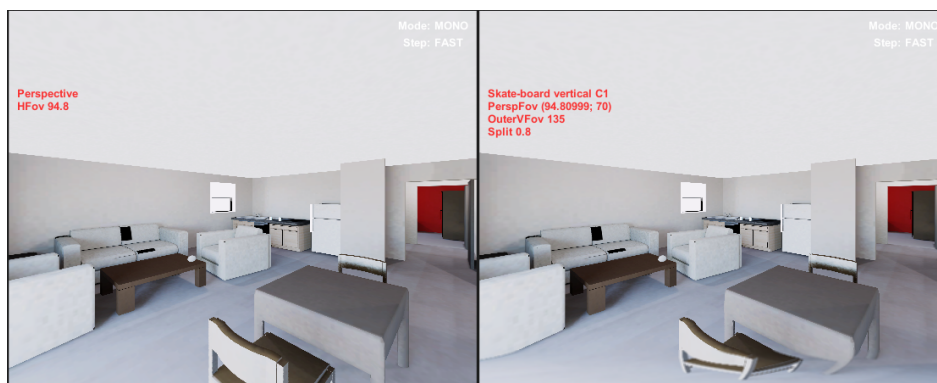
Figure 1: Left image represents a view with a perspective projection. Right image shows an example of the hybrid projection. In the left image, the user cannot see the chair behind him.
