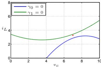
Fig. 3. Switching boundaries with spatial regularization where  $\rho = 2$ , using ( $x^* = (7, 3.27)$ ,  $E = 5\text{V}$ ,  $R = 3\Omega$ ,  $c = 0.1\text{F}$ ,  $L = 0.2\text{H}$ ,  $p_{11} = \frac{c}{2}$ , and  $p_{22} = \frac{L}{2}$ ).
