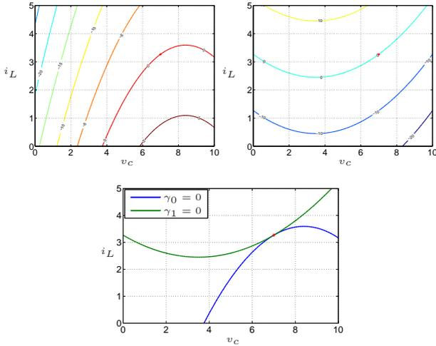
Fig. 2. Contour plots of (upper-left)  $\gamma_0$ , (upper-right)  $\gamma_1$ , and (lower) the switching boundaries  $\gamma_q(x) = 0$ , when  $x^* = (7, 3.27)$ ,  $E = 5\text{V}$ ,  $R = 3\Omega$ ,  $c = 0.1\text{F}$ ,  $L = 0.2\text{H}$ ,  $p_{11} = \frac{c}{2}$ , and  $p_{22} = \frac{L}{2}$ .
