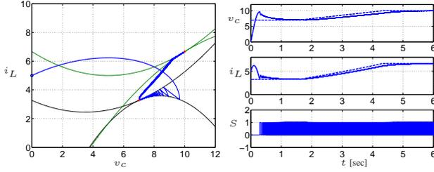
Fig. 5. Simulation results with initial conditions  $x_0 = (0, 5)$ ,  $q_0 = 0$ , when  $x^*$  linearly changes from  $(7, 3.27)$  to  $(10, 6.67)$ , where the black and green curves denote the switching boundaries for  $x^* = (7, 3.27)$  and  $x^* = (10, 6.67)$ , respectively.
