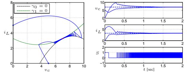
Fig. 4. Simulation results for the closed loop system  $\mathcal{H}$  with initial conditions  $x_0 = (0, 5)$ ,  $q_0 = 1$  and  $x_0 = (5, 0)$ ,  $q_0 = 0$ , and where  $S$  is only drawn for the simulation using  $x_0 = (5, 0)$ .
