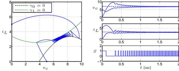
Fig. 6. Simulation results for the spatially regularized closed loop system  $\mathcal{H}^\rho$  with  $\rho = 0.5$  for initial conditions  $x_0 = (0, 5)$ ,  $q_0 = 1$  and  $x_0 = (5, 0)$ ,  $q_0 = 0$ , and where  $S$  is only drawn for the simulation using  $x_0 = (5, 0)$ .
