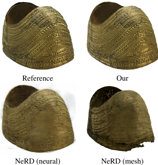
Figure 21. Example of the quality of the neural NeRD representation and their final generated mesh. Note the quality loss in both geometry and appearance (textures).
