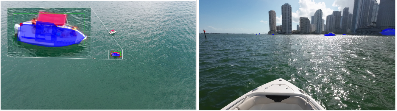
Fig. 4. Left: Example orientation of a boat taken from 50m of altitude and looking down with a pitch angle of 40^\circ . The highlighted boat has a yaw angle of 280^\circ relative to our viewpoint. Since the UAV’s heading is 170^\circ (close to true south), we know that the boat has an absolute heading of 260^\circ (close to true west). Right: Cad overlays on a frame of one the videos we took. Note the very small objects in the left part of the frame.
