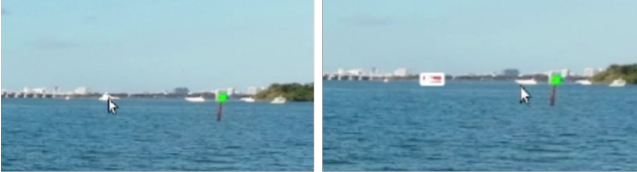
Fig. 6. Faster bounding box annotations by means of "Segment anything" [3]. We leverage this method to accelerate 2D bounding box labeling. A user just needs to click on the object, the corresponding bounding box will be set and saved automatically.
