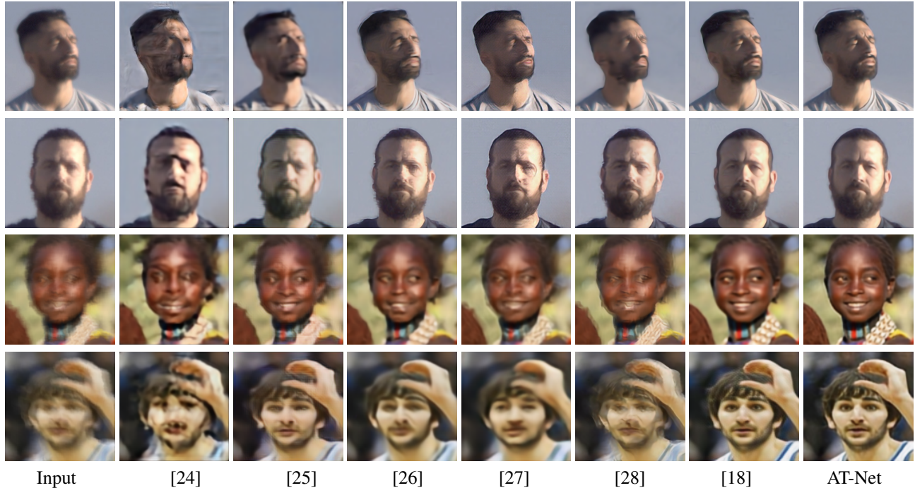
Fig. 4. Image restoration results on sample real-world (rows 1-2) and synthetic (rows 3-4) turbulence distorted images. Compared to the other methods, the proposed AT-Net method produces sharp and clean face images.
