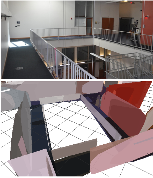
Fig. 3. The first step of this algorithm is to generate a 3-D building model which indicates the broad geometric information (but not the precise textural information). Plane colors are for illustration purposes only at this stage. This model is later used to allow an RGB-D sensor to localize.
