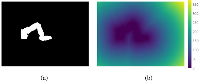
Fig. 4. Visualization of the distance map, with (a) the reference binary mask and (b) the corresponding distance map.
