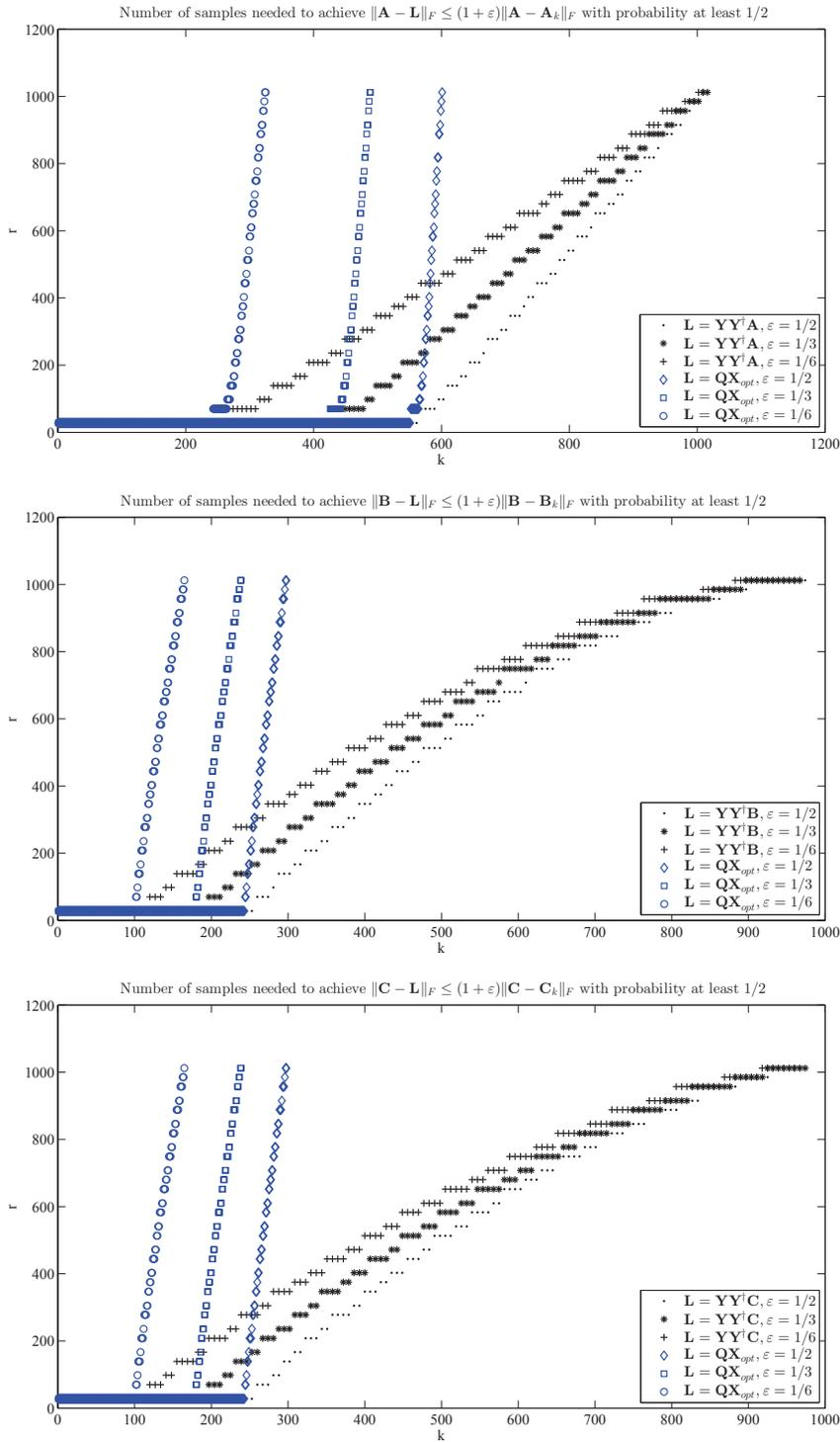
FIG. 6.3. The value of  $r$  empirically necessary to ensure that, with probability at least  $1/2$ , approximations generated by the SRHT algorithms satisfy  $\|M - YY^T M\|_F \leq (1 + \epsilon)\|M - M_k\|_F$  and  $\|M - QX_{opt} M\|_F \leq (1 + \epsilon)\|M - M_k\|_F$  (for  $M = A, B, C$ ).
