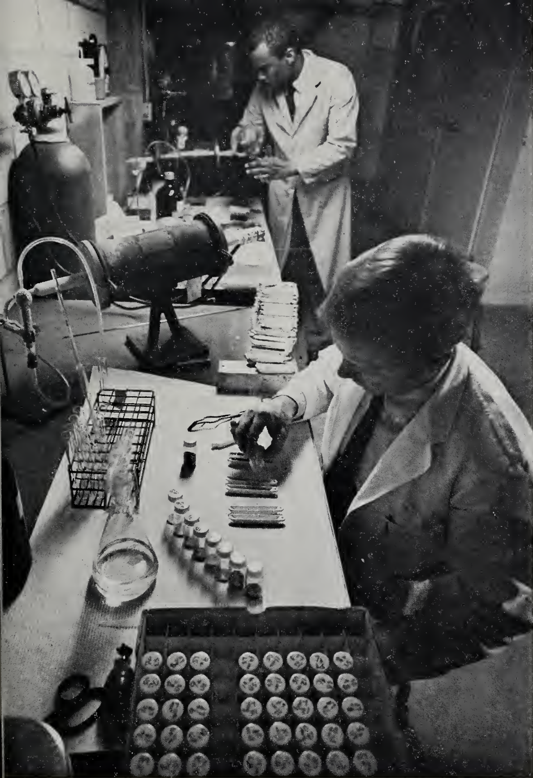
Left: Mature plants were cut and divided into stems, leaves, seeds, and pods (1269A241-24). Lower left: Beall places samples into combustion chamber to reduce samples to water, carbon dioxide, and ash. The carbon dioxide includes the radioactive carbon which is trapped in a solution. The solution is loaded into a liquid scintillation counter which measures in parts per million the amounts samples contained (1269A240-13). Below: The radioactive carbon in samples can also be counted by extracting it from the samples and then injecting the extract, as Nash does here, into a gas-liquid chromatograph (1269A242-5).
