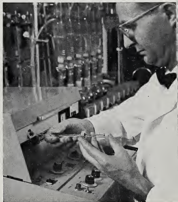
Left: Mature plants were cut and divided into stems, leaves, seeds, and pods (1269A241-24). Lower left: Beall places samples into combustion chamber to reduce samples to water, carbon dioxide, and ash. The carbon dioxide includes the radioactive carbon which is trapped in a solution. The solution is loaded into a liquid scintillation counter which measures in parts per million the amounts samples contained (1269A240-13). Below: The radioactive carbon in samples can also be counted by extracting it from the samples and then injecting the extract, as Nash does here, into a gas-liquid chromatograph (1269A242-5).
