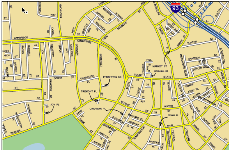
Fig. 10. Section of a city street map. Note curved leaders used to place text for small streets.
