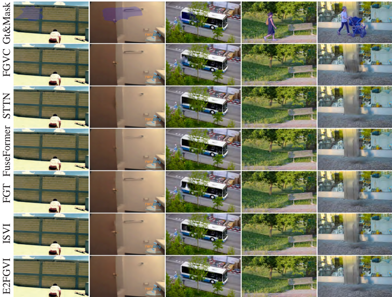
Fig. 15: Qualitative comparisons of representative video inpainting methods on YouTube-VOS and DAVIS dataset. The light blue mask highlights the corrupted regions. The first three columns are random masks and the remaining two columns are object masks.
