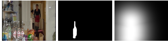
Figure 1: Example of instance: original image (programme material copyrighted by BBC), mask, saliency map generated from mask to weight the features.
