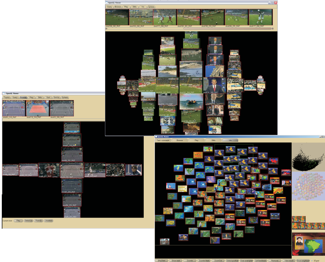
Figure 10: Interfaces of the MediaMill semantic video search engine. On the left the CrossBrowser showing results for tennis. On top the SphereBrowser, displaying several semantic threads. Bottom right: active learning using a semantic cluster-based visualization in the GalaxyBrowser.
