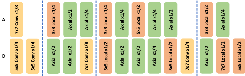
Figure 1: Searched TrioNet A and D. Conv, Local and Axial denotes convolution, local-attention and axial-attention. \times 1/2 , \times 1/4 , \times 1/8 are expansion rates. TrioNet consistently uses convolutions at low level and self-attention at high level.
