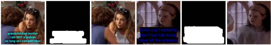
Figure 1: Selected video decaptioning results of our method. Each group includes subtitled frame, mask predicted by our caption mask extraction network, and subtitle removal result.
