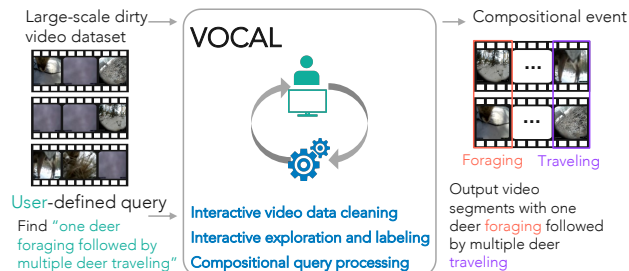
Figure 1: We introduce VOCAL, an end-to-end video analytics system that facilitates cleaning, exploration, and compositional query processing over large-scale video datasets, even for domains where no pretrained models exist.
