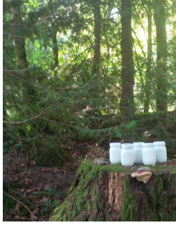
Figure 7. Example of a field trial deployment site. Devices were placed in groups of five throughout the site in simple glass enclosures.
