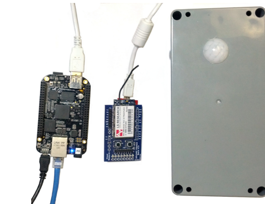
Figure 1. A gateway host (left), gateway sink radio (center), and a sensor base unit repeater in an enclosure (right).
