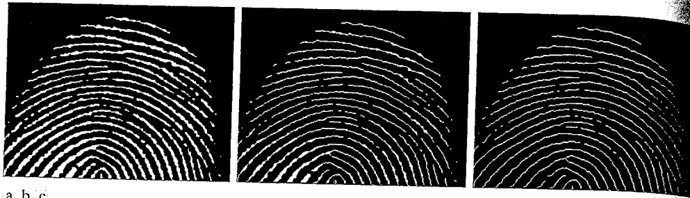
a b c FIGURE 9.15 (a) Fingerprint image from Fig. 9.11(c) thinned once. (b) Image thinned twice. (c) Image thinned until stability.
