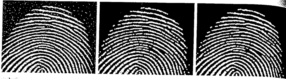
a b c FIGURE 9.11 (a) Noisy fingerprint image. (b) Opening of image. (c) Opening followed by closing. (Original image courtesy of the National Institute of Standards and Technology.)
