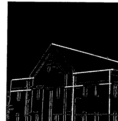
FIGURE 10.11 (a) Hough transform with five peak locations selected. (b) Line segments corresponding to the Hough transform peaks.
