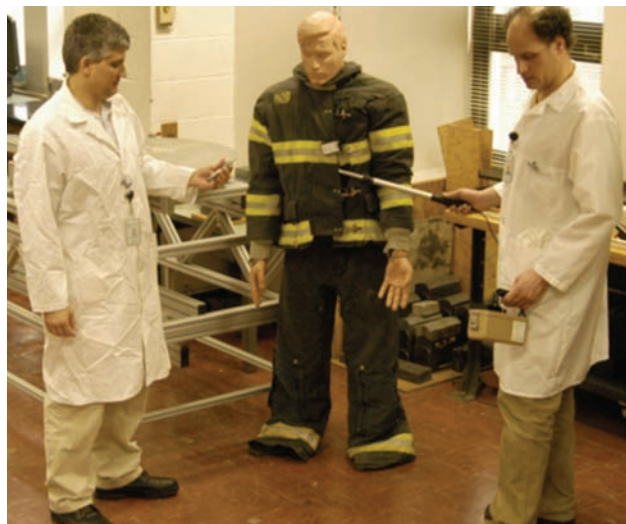
At the request of the Fire Department of New York, NUSTL scientists testing bunker gear for protection against radiation exposures.
