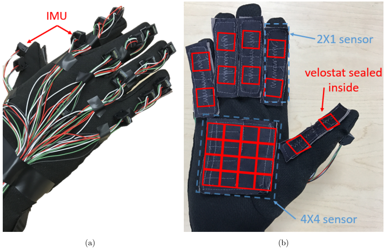
Figure 2.1: Prototype consisting of (a) 15 IMUs on the dorsum of the hand and (b) 6 integrated Velostat force sensor with 26 taxels on the palmar aspects of the hand.
