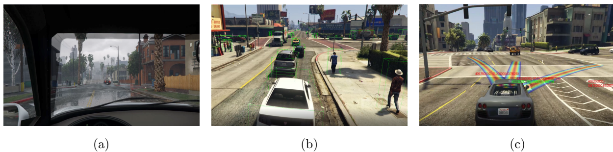
Figure 5.4: Sketch of autonomous driving in GTA game. (a) Weather control for road conditions. (b) 3D bounding boxes information extracted for on-scene agents. (c) Heatmap predictions for driving maneuvers.
