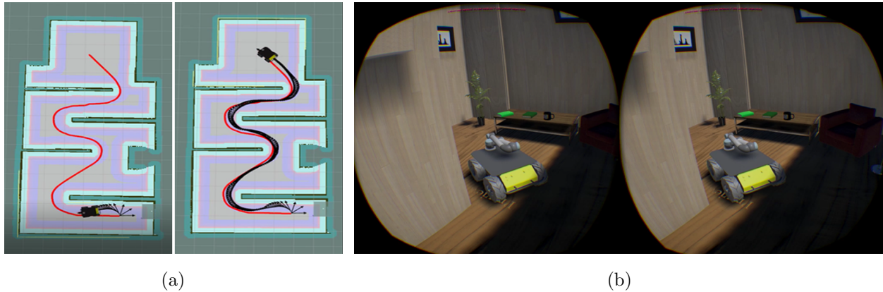
Figure 3.6: VRGym-ROS bridge. (a) The robot navigation in the scene imported into the Gazebo, exported from the VRGym. The red curve indicates the path planned by the robot’s global planner. The black curve is the actual trajectory executed by the robot. (b) A Husky-UR5 robot is imported into VRGym from ROS to guide the way and open the door for a human agent.
