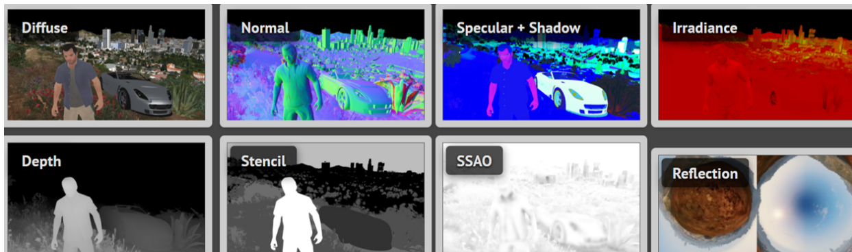
Figure 5.2: G-Buffer shading results on GTA game. The pixel shader fetches data from different combination of buffers and compute the final shading value of the pixel in HDR. Visual ground truth such as depth and instance segmentation are obtained by hooking with the rendering process.
