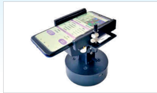
A prototype of microscopic image based vegetable quality assessment system
