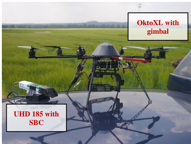
Figure 2: UHD 185 with SBC and OktoXL with gimbal
