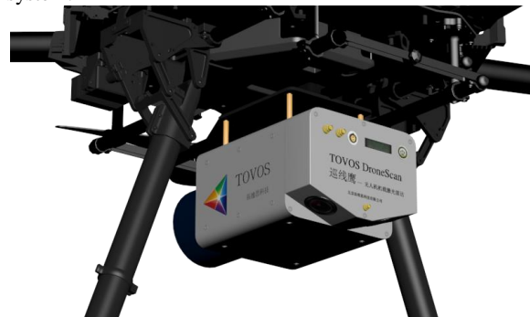
Figure 2. Tovos DroneScan mounted on DJI M600 pro
