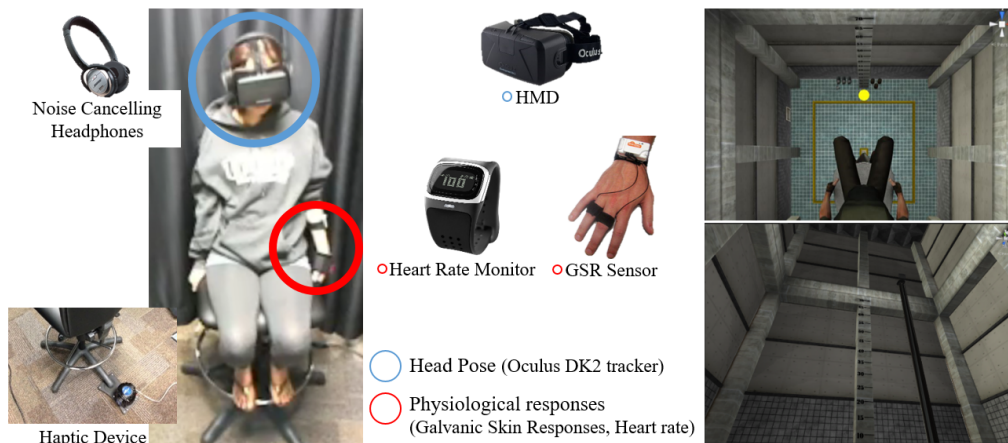
Figure 3: Virtual pole setup used in Experiment 2. A stool without armrests was used to increase instability. A haptic device was attached to a leg of the stool to simulate mechanical vibrations. Participants were exposed to the IVE (images on the right) using the Oculus DK2 HMD and a noise cancelling headphone. During the simulation, their physiological responses and head motion were recorded.
