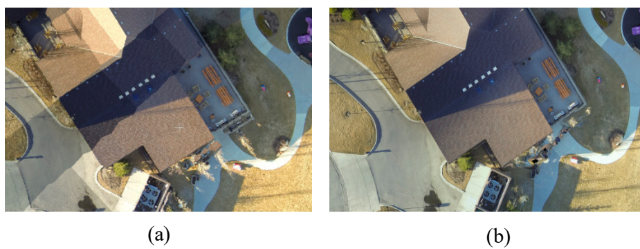
Figure 16. The generated RGB-based orthophoto mosaic from (a) the proposed automated aerial triangulation, and (b) Pix4D for Phantom2-Building Dataset.
