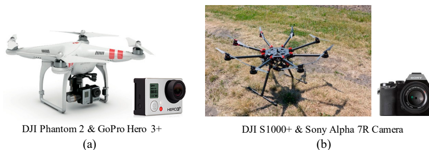
Figure 11. (a) The DJI Phantom 2 UAV with a GoPro Hero 3+ camera mounted on a gimbal, and (b) the DJI S1000+ UAV equipped with a Sony Alpha 7R camera with a vertical view.
