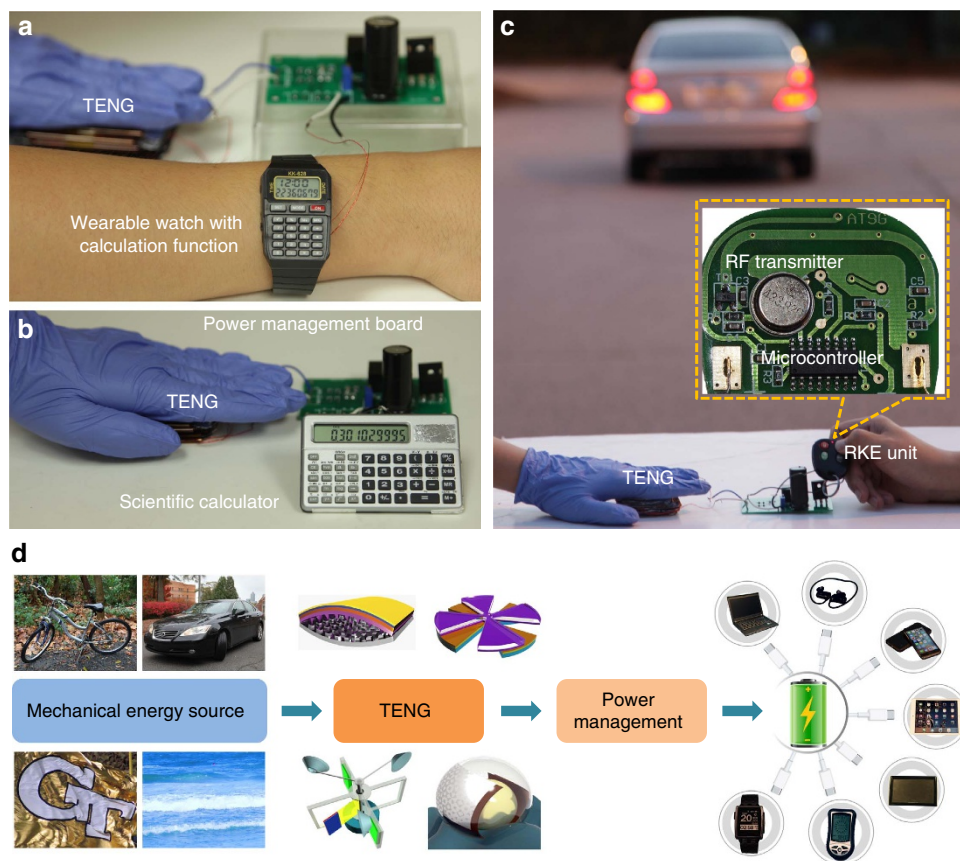
Figure 4 | Application in self-powered data-processing and transmission system. (a) Demonstration of a self-powered wearable watch and calculator. (b) Demonstration of a self-powered scientific calculator. (c) Demonstration of a self-powered RKE system. (d) Extension of this TENG-based self-charging unit for various applications as a universal adaptable power source.
