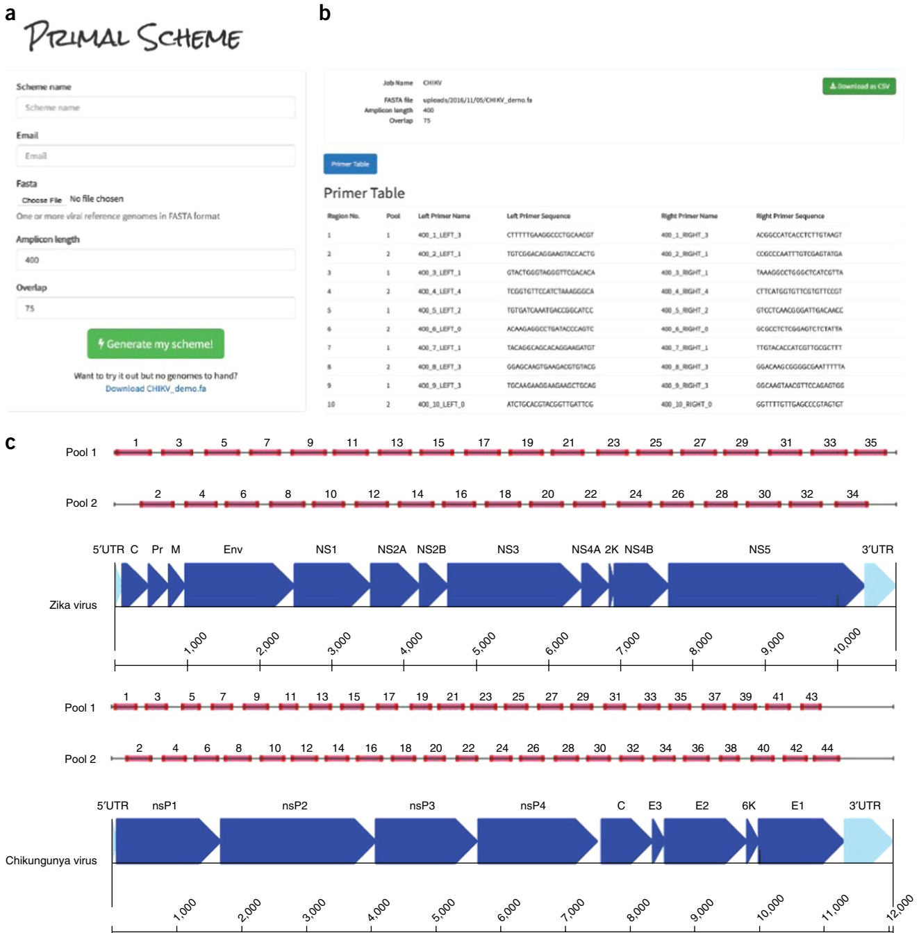
Figure 2 | Overview of multiplex primer design using Primal Scheme online primer design tool. (a) Submission box for online primer design tool. (b) Primer table of results. (c) Schematic showing expected amplicon products for each pool in genomic context for the ZikaAsian and ChikAsianECSA schemes.
