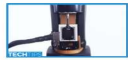
Installation & Calibration of the Relative Humidity Accessory for the Discovery Hybrid Rheometer
