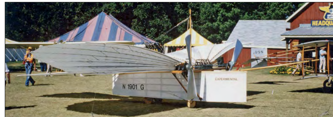
ABOVE In the 1980s–90s two flying "replicas" of the Whitehead No 21 were built, one in Germany and this one, designated "No 21A", in the USA. Although both were flown, structural and aerodynamic differences, plus the use of modern powerplants, mean that they cannot be regarded as proof that the original aircraft was capable of flight.
