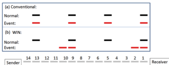
Figure 2. Conventional approach vs. WIN. Time slots labeled by time are shown at the bottom. Solid bars denote normal (black) and event (red) packets transmitted at various time slots.
