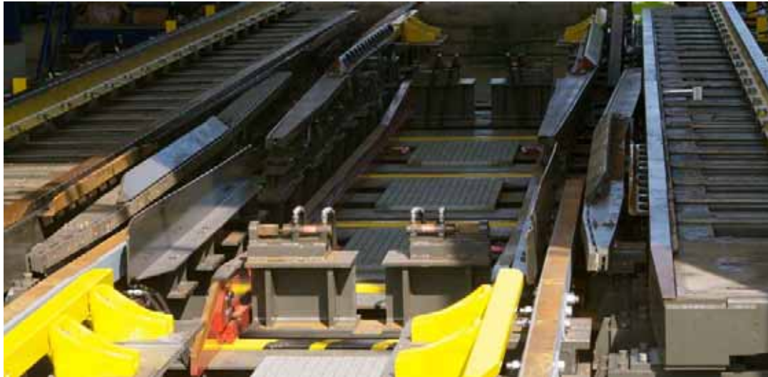
Test changer TCRS3 in the CAF position. Notice that the Talgo locking devices have been lowered and the guide rails have been moved sideways.
