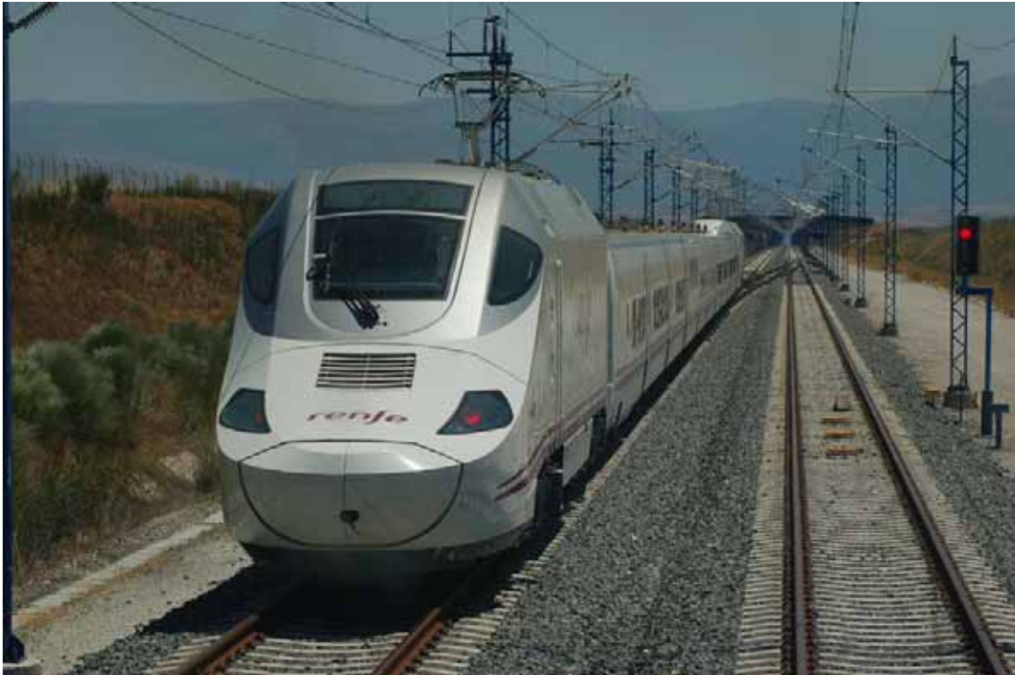
Talgo series 130 variable gauge train on high-speed line
