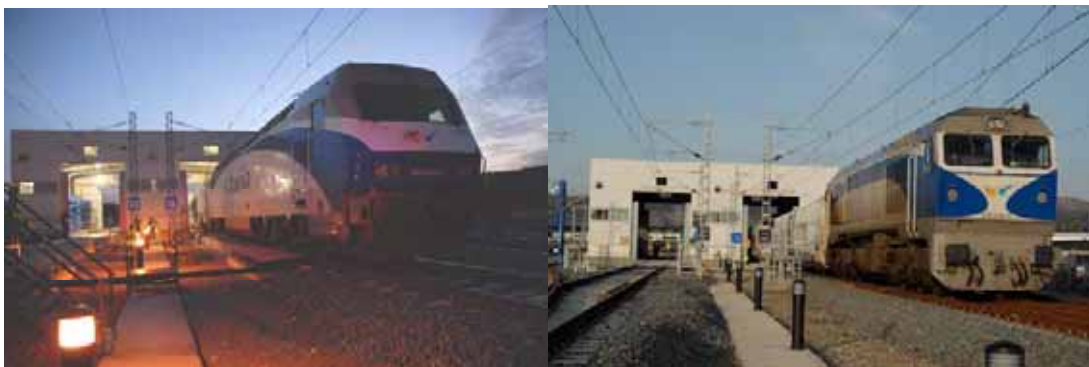
At Antequera Santa Ana there are two dual changers (CAF and Talگو) that are used for the Madrid, Algeciras and Granada trains
