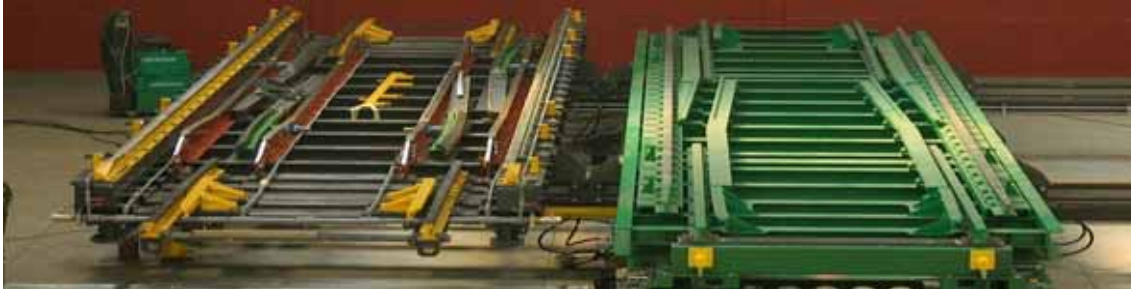
The third generation changers are versatile and the platforms are superimposed on a bedplate, instead of embedded in a pit. The photo shows a Talgo platform on the left and a CAF platform on the right.
