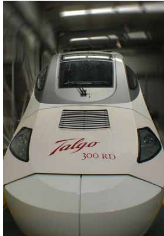
Power car of the Talgo variable gauge prototype capable of reaching 300 km/h. CAF has announced the launch of a similar train.
