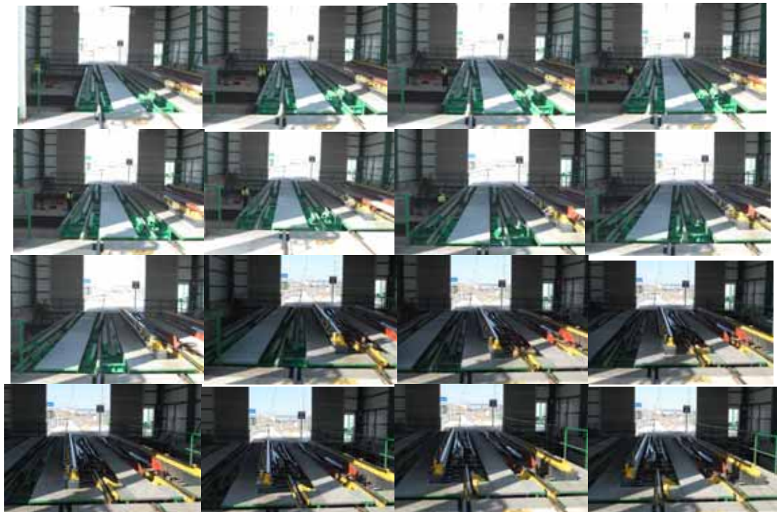
Sequence of steps involved in changing from CAF platform (top left) to Talgo platform in a horizontal changer, in this case Valdestillas. (Photos: Ana López Romero)
