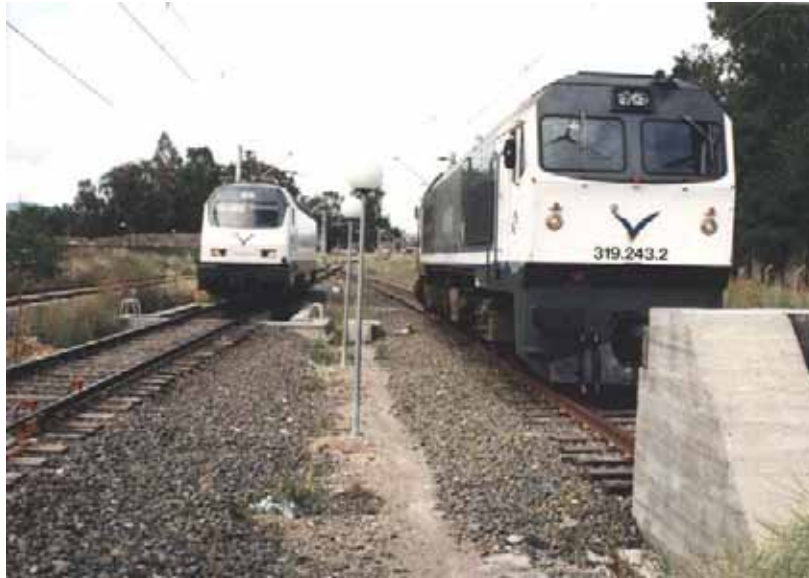
In the second-generation gauge changers, it is necessary to change the locomotive. The photo shows an electric locomotive 252 and a diesel locomotive 319 passing through the Córdoba gauge changer (1994).
