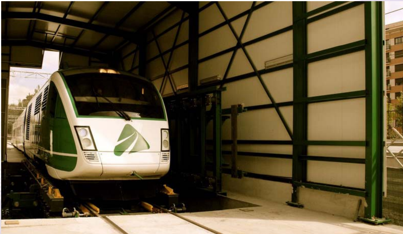
Gauge change shunting with ADIF's BT Diesel train
