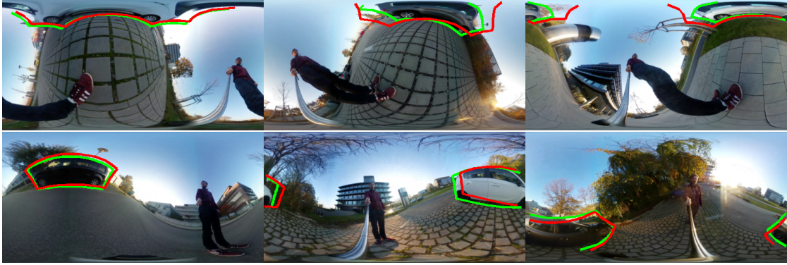
Figure 4.10: Detection Results on OmPaCa Dataset. The ground truth is shown in green, our SphereNet (NN) results in red.
