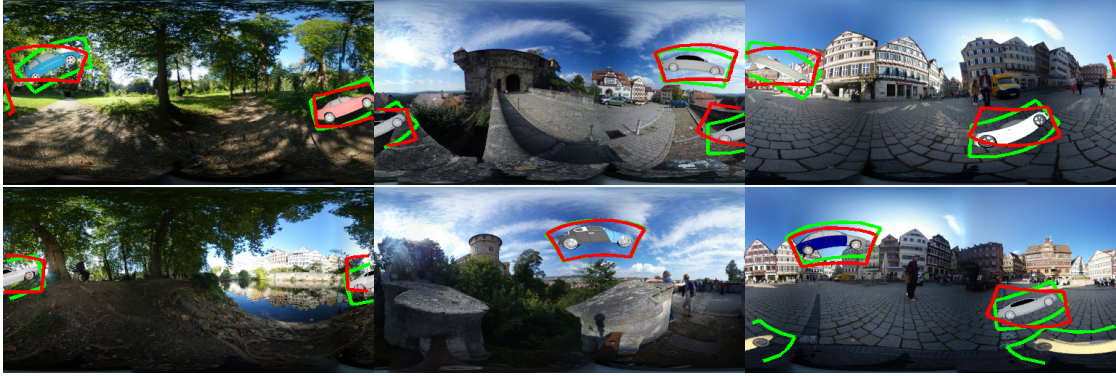
Figure 4.9: Detection Results on FlyingCars Dataset. The ground truth is shown in green, our SphereNet (NN) results in red.
